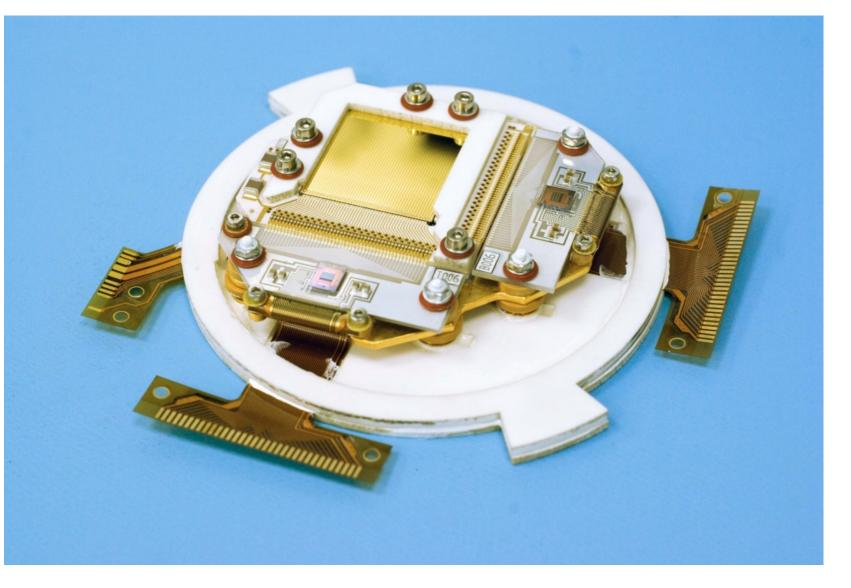
Each ART focal plane detector (*above*) is held within a ceramic housing along with front-end electronics (ASICs) located on two edges that are coupled to flexible circuit boards. Spectral resolution
