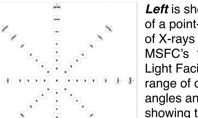
*Left* is shown images of a point-like source of X-rays captured at MSFC's 104 m Stray Light Facility at a range of off-axis angles and azimuths showing the 0.5'
